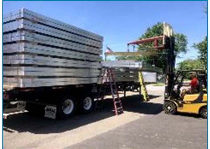
Aluminum reactor cages for PECO required over 2,100 hours of fabrication in the shop.
