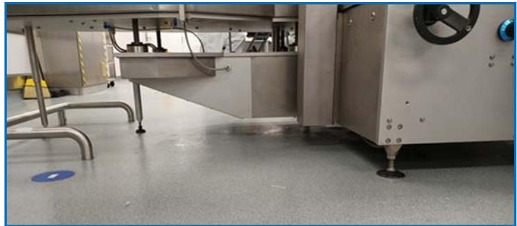
Menold's design team measured the space of the existing equipment, ensuring their skirting solution would fit snug against all the components.
