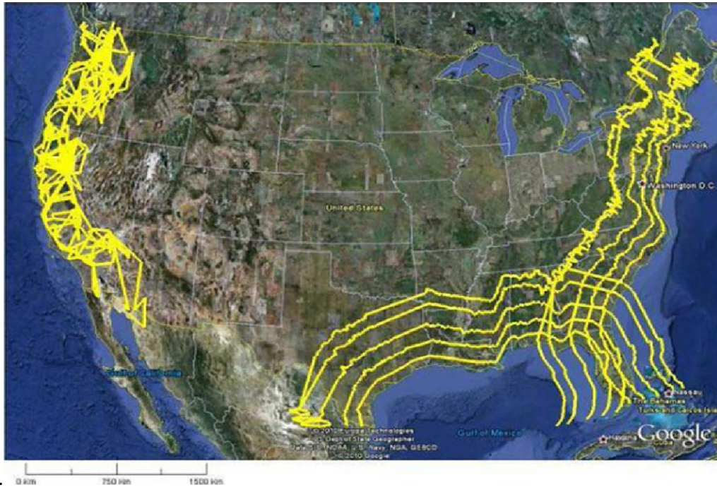
NTIA map depicting a composite view of the exclusion zone distances for different shipborne radar systems, as set forth in the NTIA’s 2010 Fast Track Report. 19
