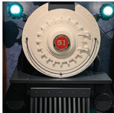
Featured (left) is a scaled down version of a steam locomotive boiler front with steam chests, cowcatcher, original head light, marker lights and a Baldwin builder plate.
