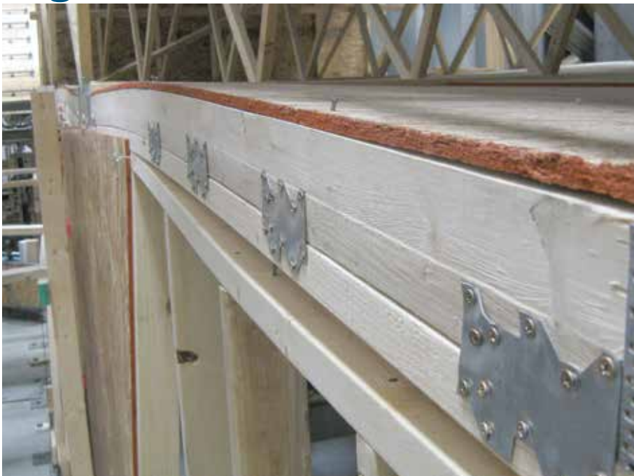
In practice, ASTM E72 causes severe stress on the corner connectors of a wall.
