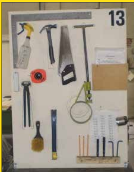
When taking the "5S" approach to dealing with making your production areas more efficient, one idea to consider is creating Kaizen boards to organize tools.
