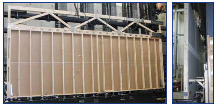
Figure 1: Photos of ASTM E2126 Test Setup with Gypsum Shear Wall.
