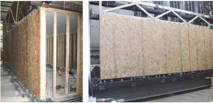
Figure 6. 12'x30' Building vs. Lateral Wall Station w/ Truss Test Setup for Fully-Sheathed WSP Shear Wall
