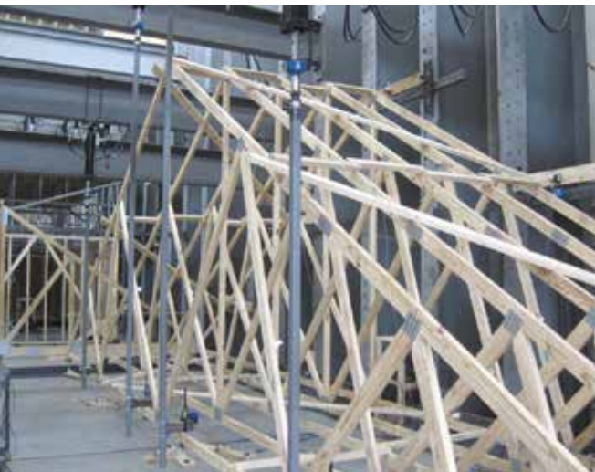
Full-scale assembly set-up tested at SBCRI.
