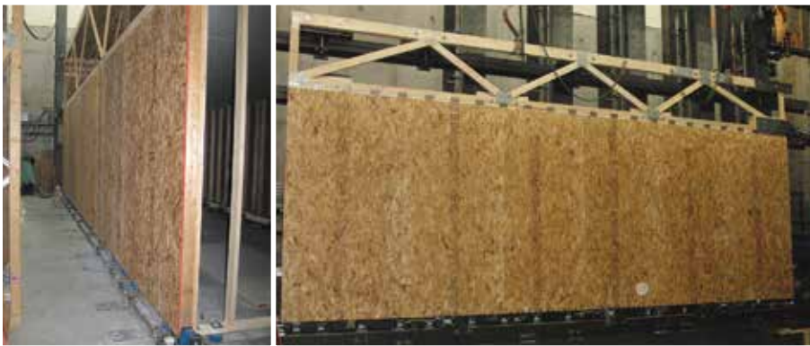
Figure 4. Fully Sheathed Wall Testing: The results from the 12' x 30' full building lateral wall with a full set of roof trusses test were compared to the lateral wall station with truss framing tests to ensure they produce similar results.
