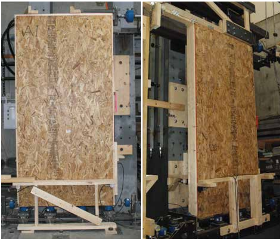
Figure 2. Single Panel Wall Testing: The results from these two single panel wall test setups were compared to ensure they produce similar results.
