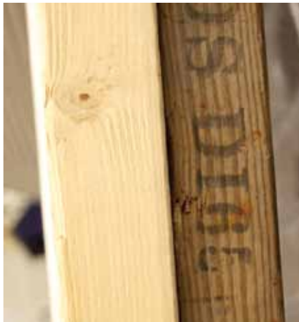
Photo 1. While No. 2 lumber (left) and scaffold-grade lumber (right) may look similar at first glance, scaffold lumber meets a number of particularly high standards, which most construction-grade lumber does not meet.
