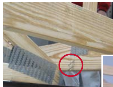
A2 fails when the truss pulls out from the two end nails girder during Test 1. No hanger is present. Compare to jobsite failure in photo below.
