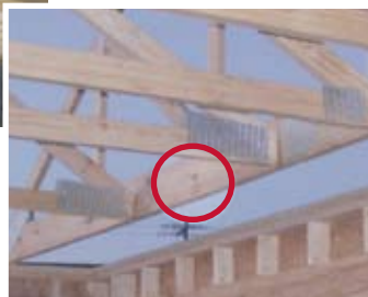
A2 fails when the truss pulls out from the two end nails girder during Test 1. No hanger is present. Compare to jobsite failure in photo below.
