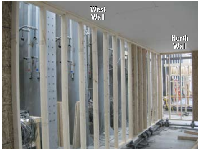
Photo 6. In the first baseline IRC test, no gypsum was applied on the inside of the 30' wall. This was our approach to replicate the IRC defined 500 plf and AF&PA's SDPWS 515 plf braced wall panel design.
