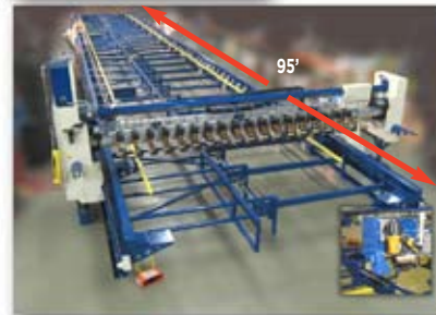
• Custom built 95 feet of expanded wall panel capability with Dual Tool Beam and Dual Top & Bottom Nailers (builds up to 76' wall)
