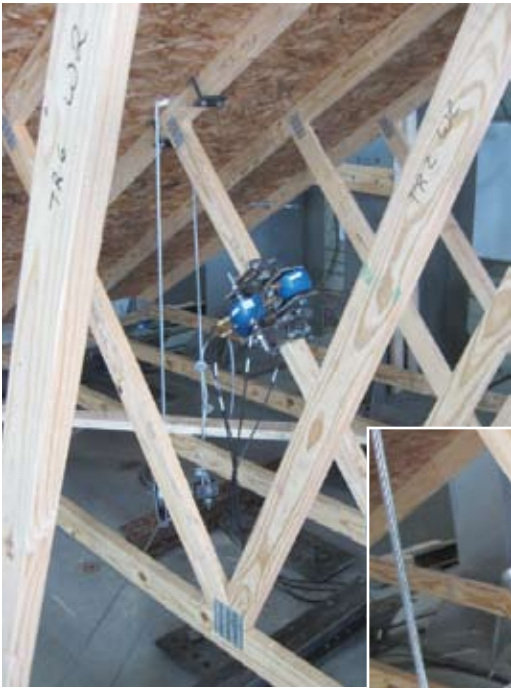
Figures 11 & 12. WB3 is used to test the forces through a web in a full-scale assembly.
