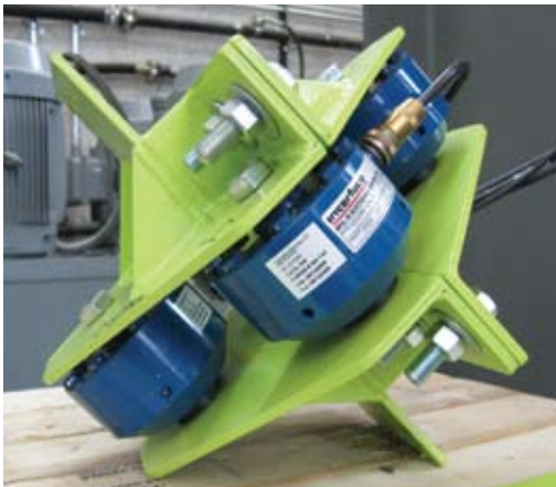
Figure 4. Adding two load cells to WB2 allowed forces to be measured on the top and bottom axes.
