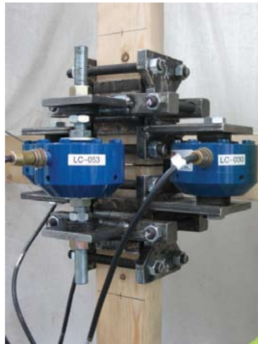
Figure 9. Changes made to WB3 were intended to stabilize the web and improve load transfer.
