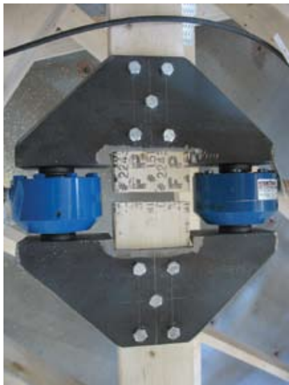
Figure 1a. "Web brace" 1 is attached to a web with bolts. Two load cells (in blue) measure forces running through the web.
