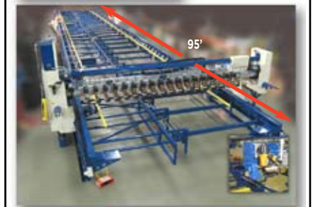
• Custom built 95 feet of expanded wall panel capability with Dual Tool Beam and Dual Top & Bottom Nailers (builds up to 76' wall)
