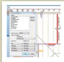
Pinpoint and replace any wall member using TrussFramer's Search and Replace tool, making changes to lumber grade, species, size, or type quick and simple
