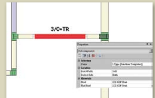
With Plan View Panel Editing, easily edit wall panel members and subcomponents directly from plan view. This overhead view lets you see all related walls and understand how they interact with one another.
