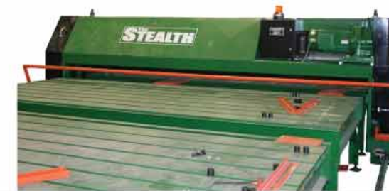
24" Gantry on Crane Rail
