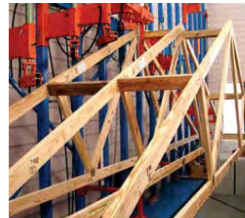
Fig 3. Test II configuration of three 24-foot span Fink trusses interconnected with 2x4 short member lateral restraint.
