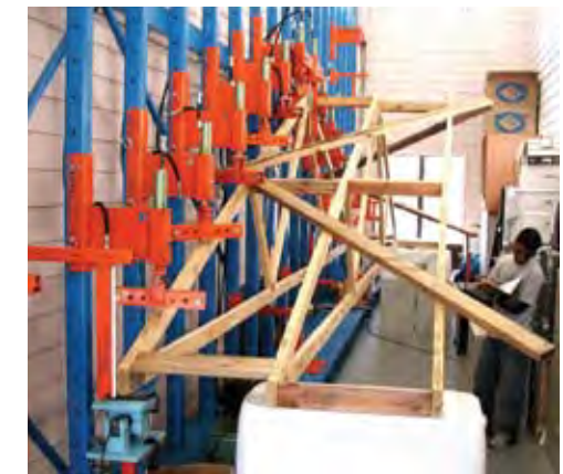
Fig 4. Test III configuration of three 24-foot span Fink trusses with 2x4 short member lateral restraint and diagonal bracing.
