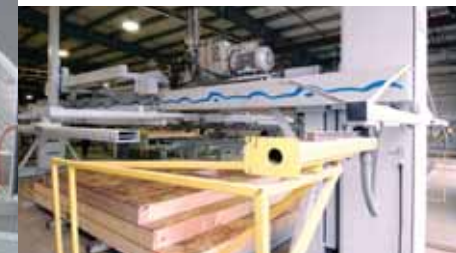
Automated Panel Stacker
