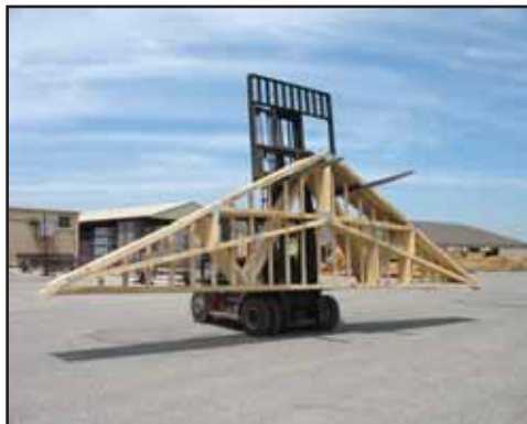
Keeping forks low to the ground and operating the lift at a reasonable speed will minimize the potential for danger.
