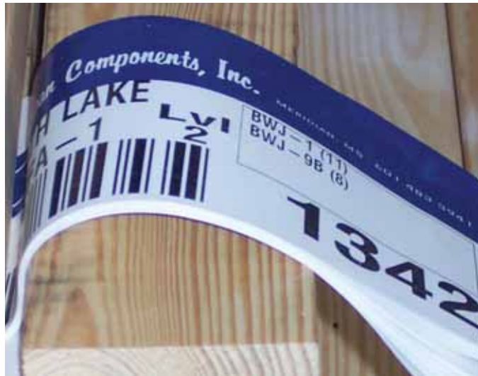
Job identification tags stacked on cart before truss assembly.
