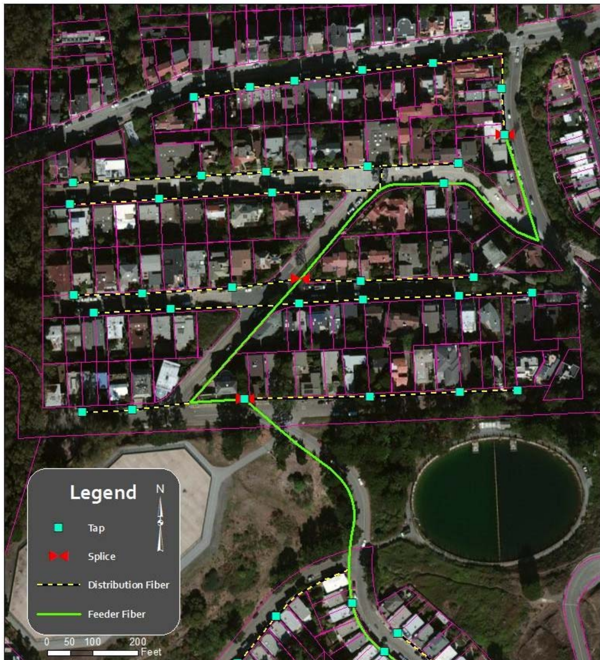
Figure 8: Sample FTTP Access Layer Design
