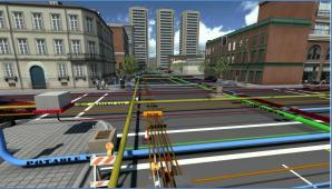
The illustrations above show tidy diagrams of what is usually not at all clear or straightforward as a contractor cuts and trenches along the roadway.<sup>25</sup> These diagrams don't take into consideration rural America underground, which will likely include culverts, drainage systems, septic tank pipes, and agricultural infrastructure such as irrigation systems.
