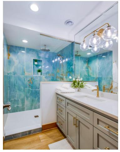
A glass partition separates the space without a shower door, requiring the entire area outside the shower to be waterproofed. For safety, the pony wall is anchored with metal angle supports.
