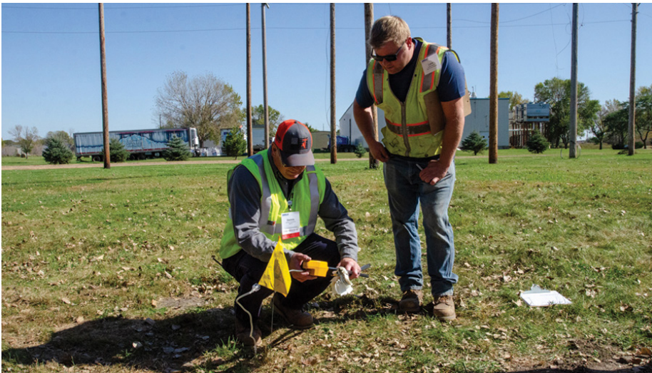
Bill Gustafson from Fosston watched as a leak field investigation was carried out. Here, a hole is drilled into the ground where a CGI is inserted, which, when using the bar hole function, informs the user of the underground gas leak concentration.
