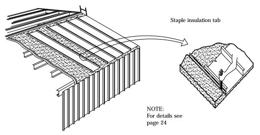
Place panel from stack onto the insulation to hold in place while stapling the joint.
