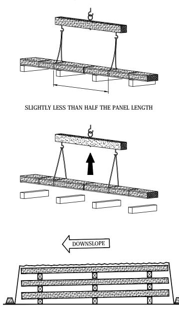
When using a crane and wire rope sling, examine the wood crating to make sure the wood prevents the slings from damaging the panels. Nylon slings are necessary when handling crates that have been opened or no longer have the wood crating for protection. The distances between the slings should be a little less than half the length of the panel.
