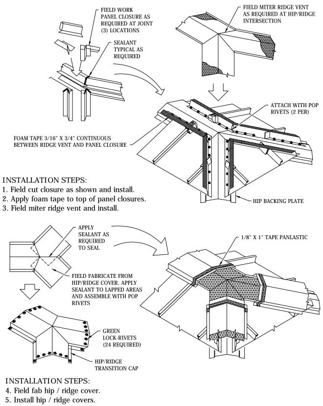
6. Apply tape Panlastic to top of hip / ridge covers to receive hip / ridge transition cap.
