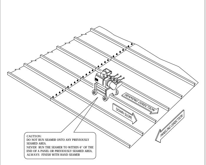
FOR ROOF WITH PANEL SPLICES In-line panel splice shown. Method for seaming staggered splice procedure is identical see important note below.
