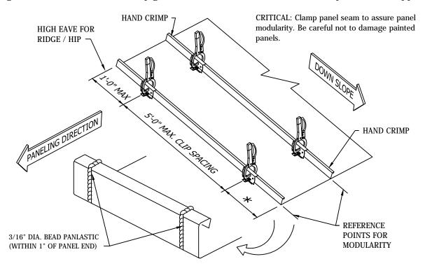
Make sure panel module falls on marked reference points. Make certain that previous seam is tight and adjacent roof clips are tight against male hem before securing with fasteners. Use clamp as shown.
