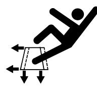
Never step on a single roof panel or a stack of several roof panels lying unattached on the roof structurals. If you step onto a single panel lying unattached on the roof structurals, it may slip causing you to lose your balance and fall. Even a stack of several panels lying unattached on the roof structurals may slip if you step on it.
