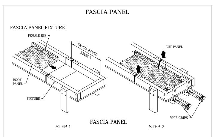
Determine and measure distance from end of panel to bend point, marking each high rib. Cut the upper flange and vertical leg of high rib to start of radius corner using a hand band saw.
