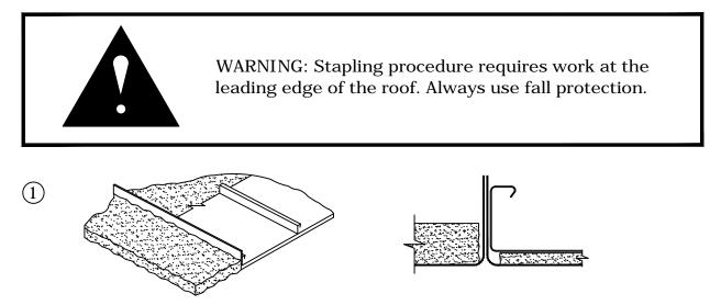
Stapling is done from the topside as the insulation is applied. Pull the adjoining facing tabs outward at the joint and align the top edges of the two tabs.
