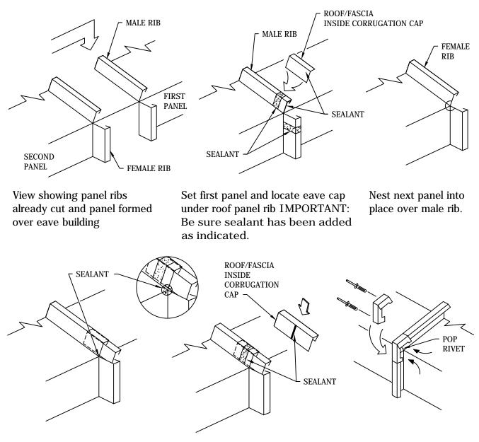
Completed view of panels nested together. Proceed with seaming operation after panel clips and panel attachment fasteners have been located.
