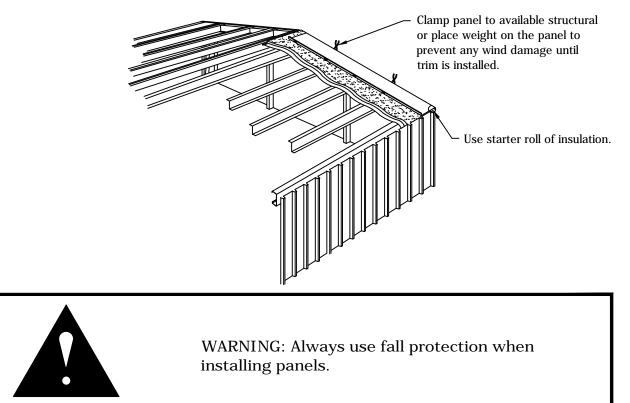
To install the first panel, field cut and position the right hand edge of the panel at structure line.
