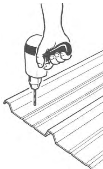
DRILLING 1/8" HOLES AT CENTER PUNCH LOCATIONS
