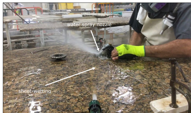
A worker uses an angle grinder with a diamond grinding cup wheel to finish a stone countertop. Combining “sheet-wetting” with a water spray nozzle helps reduce RCS exposure during grinding. Photo by NIOSH.
