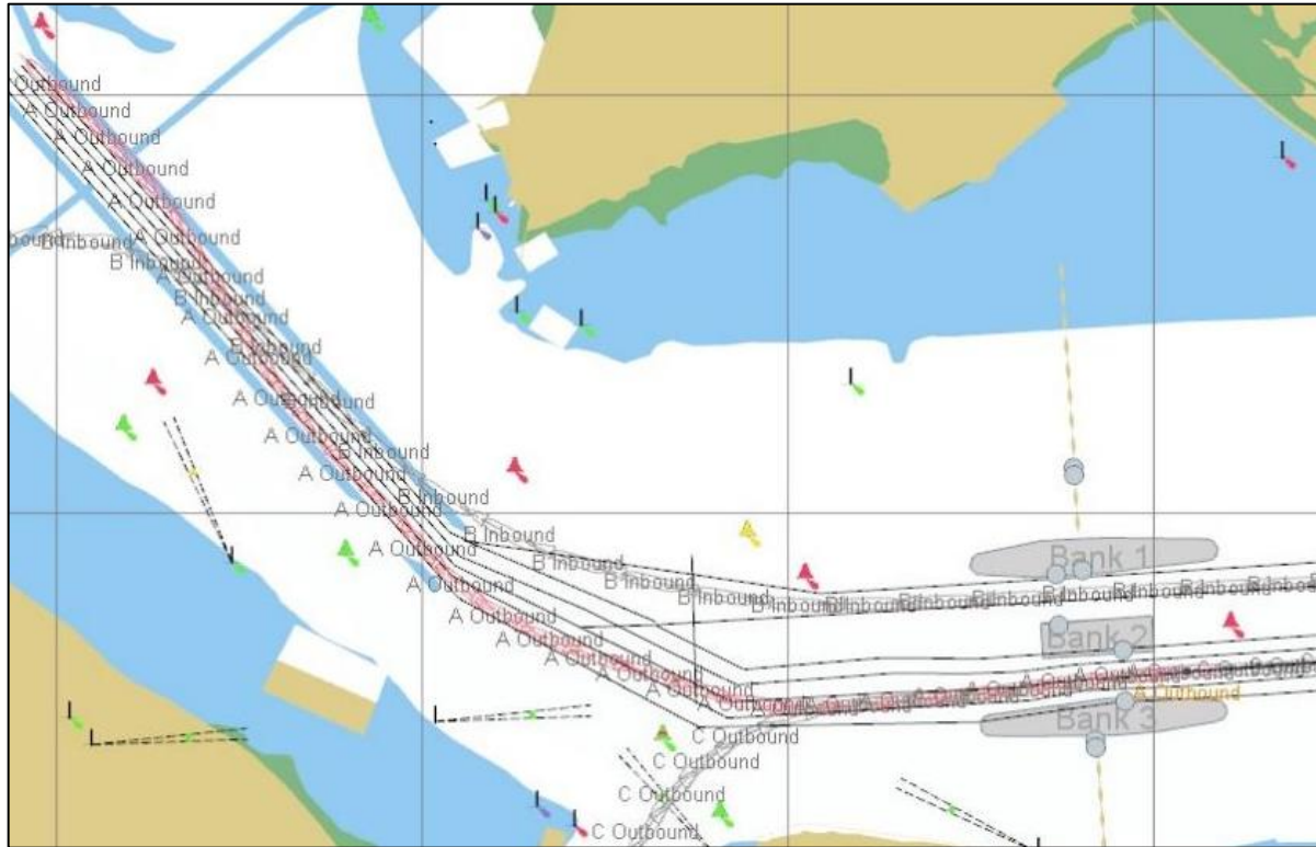
Figure 16. Run #31, outbound ship has flood current, could not get aligned with gates after turn at buoys 18 and 16, entered gate system at an angle
