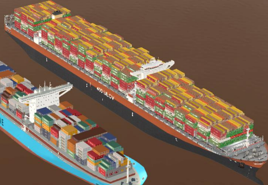
Near Future Vessel 21,000 Container Capacity 1300' long x 177' wide
