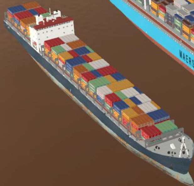
Existing Vessel 6,000 Container Capacity 964' long x 106' wide
