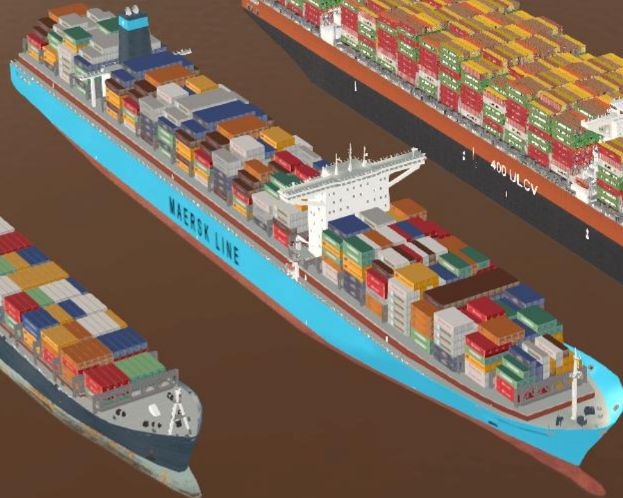
Existing Vessel 6,000 Container Capacity 964' long x 106' wide
