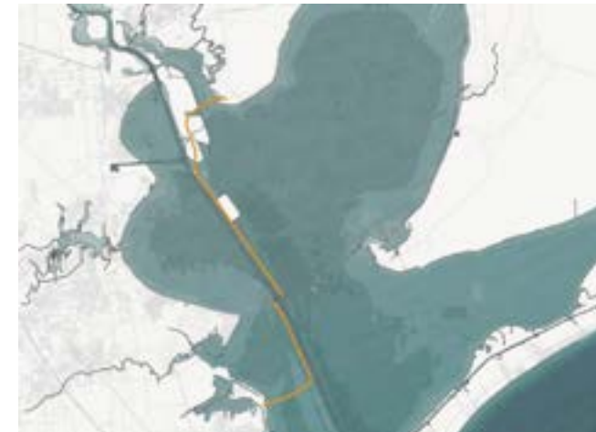
Figure 1. Layout of 25-foot barrier adjacent to the Houston Ship Channel. Image by Rogers Partners Architects for SSPEED Center.
