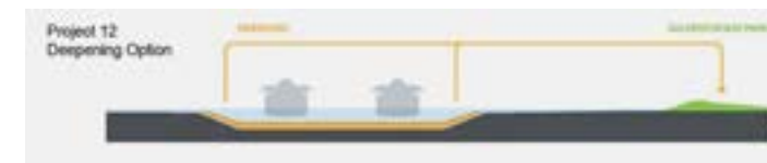
Figure 2. Diagram illustrating use of Houston Ship Channel dredged material for levee construction. Image by Rogers Partners Architects for SSPEED Center.
