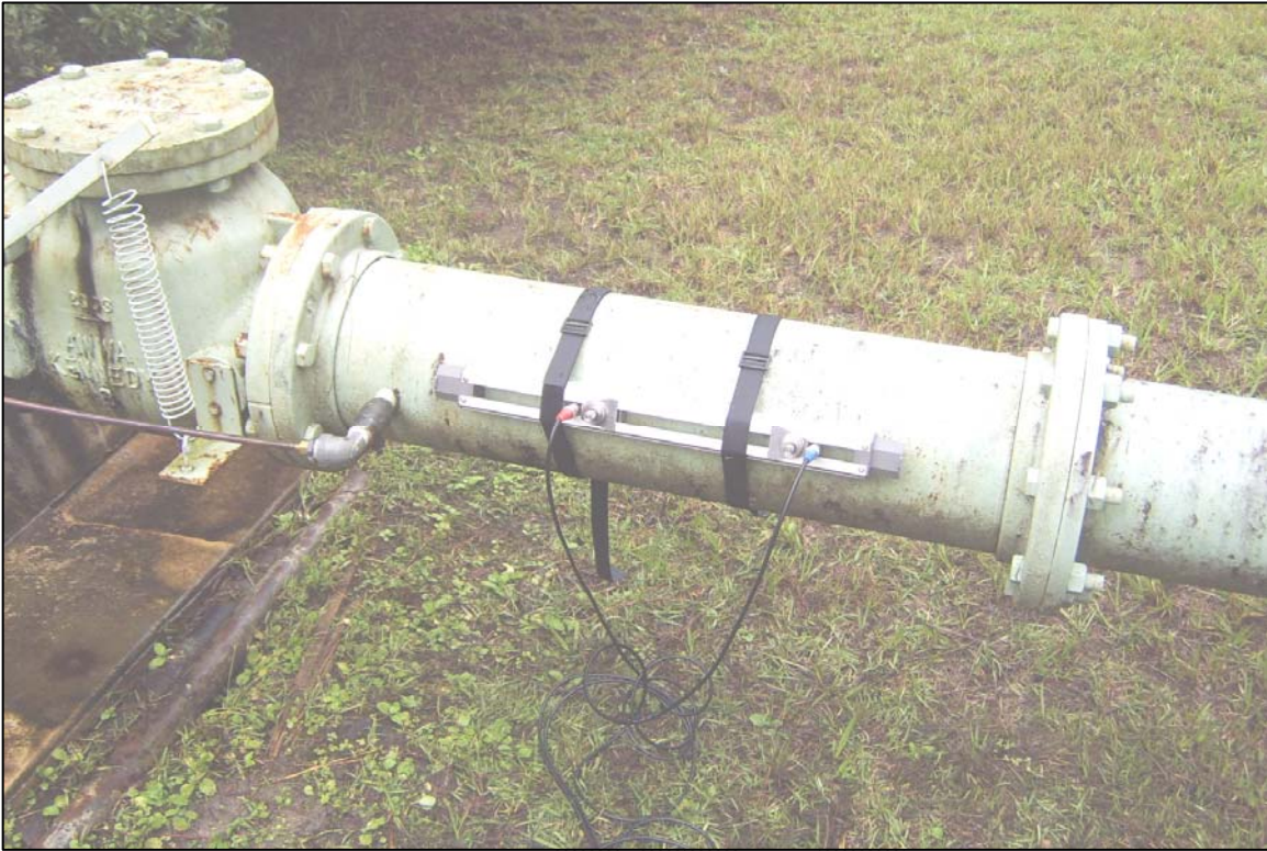
Strap-On Ultrasonic Meter for Calibration
