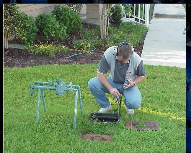
Leak Detectors Used to locate water leaks by sound amplification.
