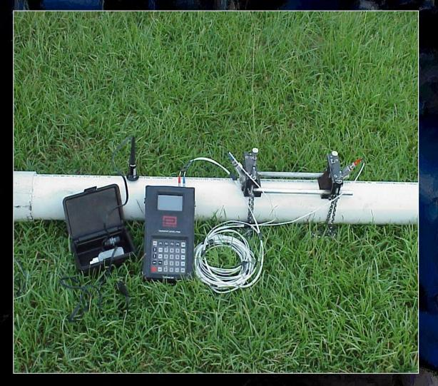
Panametrics Ultrasonic Flow Meter Used to test meter accuracy and provide flow data on water systems.
