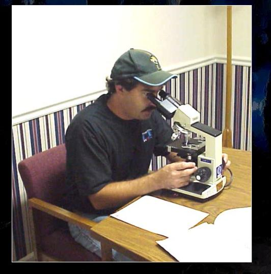
Microscope Observe mixed liquor samples for process control analysis.
