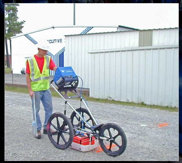
Ground Penetrating Radar Radar Helps locate underground pipe (metallic and non metallic)
