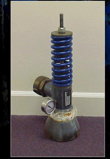
**Pressure Relief Valve** Used on hydrants or blowoffs to relieve excess pressure on water lines.
