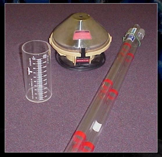
Sludge Judge measure sludge depth Settleometers test mixed liquor settle ability • Centrifuge spins and makes bugs dizzy
