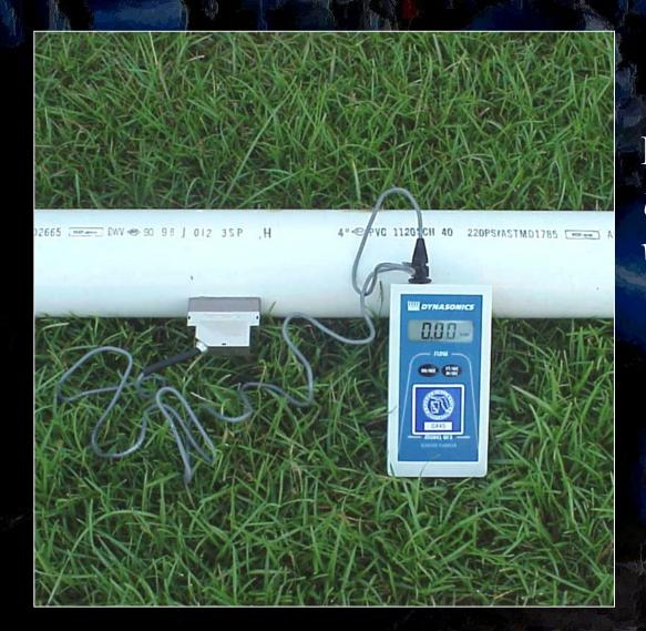
**Doppler Flowmeter** Used to measure velocity of wastewater flow.
