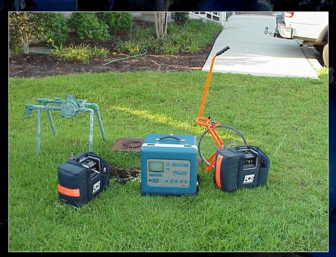
Computer Leak Detector Correlator Used to pinpoint water leaks by sound amplification.
