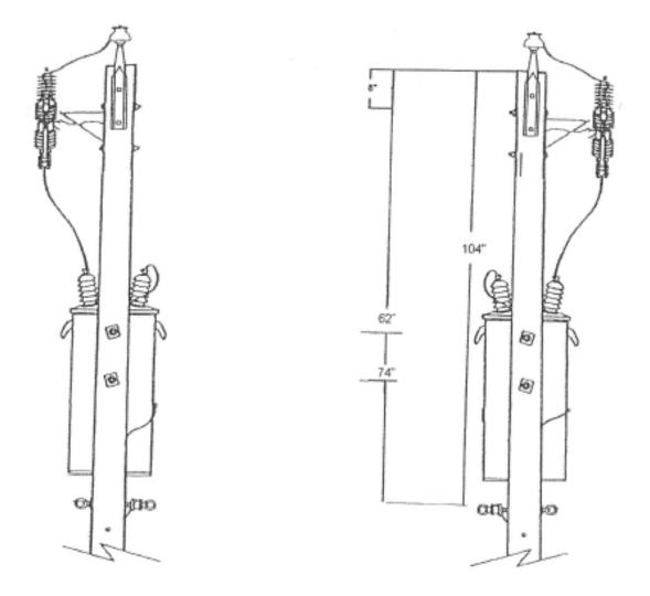
Above is a view of how either station will be built. If the station is built as the left drawing or the right drawing, the other station will already be built as shown minus the cutout door and transformer. Poles will be set approximately 4 feet apart.
