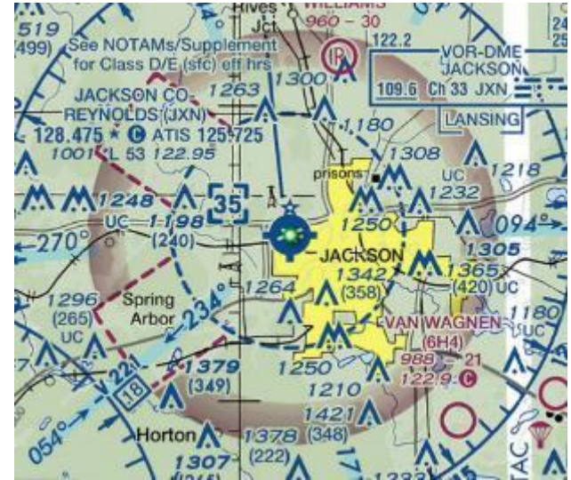
Clip of FAA Visual Flight Rules (VFR) Aeronautical Chart for Detroit showing the Jackson area.
