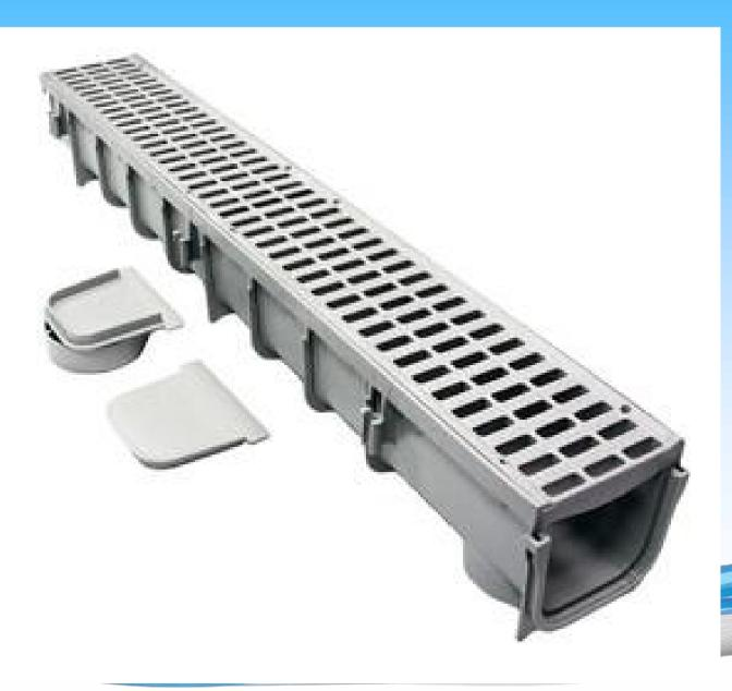
**Plastic Drains** expand when hot liquids a run into them. The sides of the drains pull away from the substrate. No amount of caulk will solve the problem
