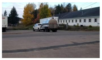
capabilities. Direct fill operations utilize insulated milk transport trailers for storing the milk until it leaves the farm. These type of storage units function as a thermos bottle to store the milk. They do not have agitation or cooling capabilities, and milk loaded onto trucks during milking must be properly cooled before loading.
