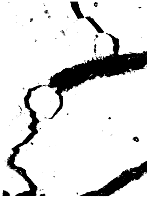
Micrograph of Gray Iron showing crack-life behaviour of graphite flakes.
