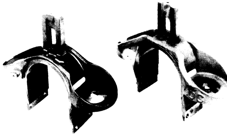
Railway axle-spring adaptor (by courtesy of SKP Sweden). Left: ADI (Muhlberger GGG100B/A). Weight: 29,7 kg. Right: SG iron GGG80. Weight: 42 kg. Weight savings with ADI = 12 kg (30%).
