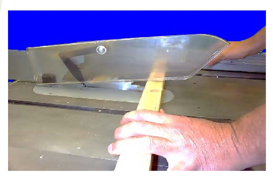
Table saw MUST be guarded by a hood which shall completely enclose the portion of the saw above the table.
