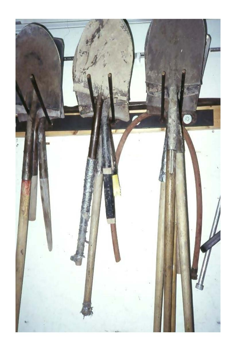
The wooden handles of all tools shall be kept free of splinters or cracks and shall be kept tight in the tool.
