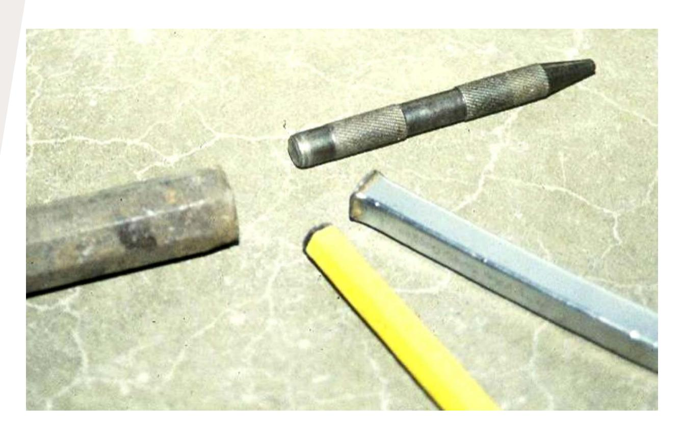
Impact tools, such as drift pins, wedges, and chisels, shall be kept free of mushroomed heads.
