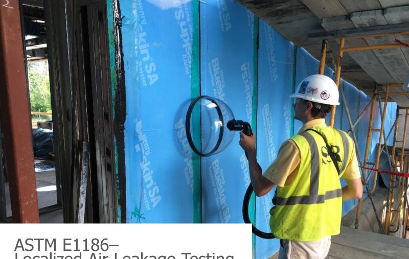
ASTM E1186– Localized Air Leakage Testing "Bubble Gun"
