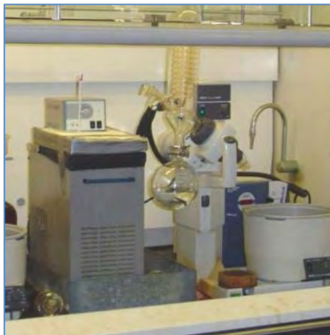
Figure 7.55 - Recirculating Refrigeration System in a Chemistry Laboratory
