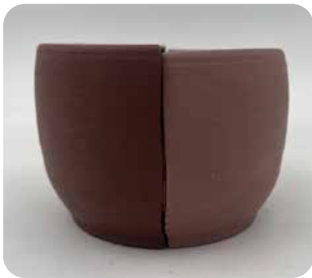
You can see the difference in the color of the clay and the shrinkage from leather-hard (left) to bone dry (right).
