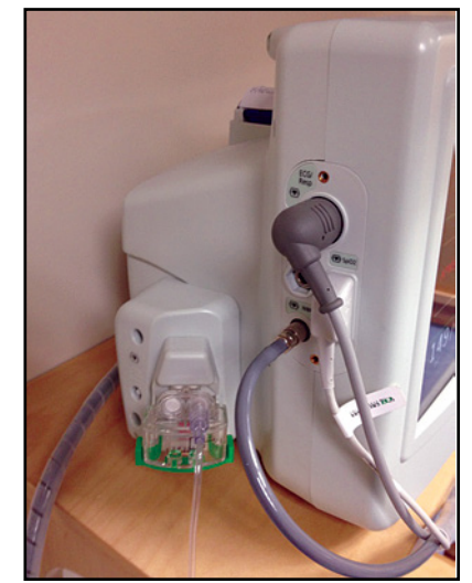
Figure 12. Built in moisture trap and filtering capnography coupler on a multiparameter monitor
