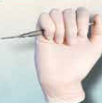
Blade Holder with Drop Control Eject used blades by pressing button at end of blade holder. Eject with one hand.
