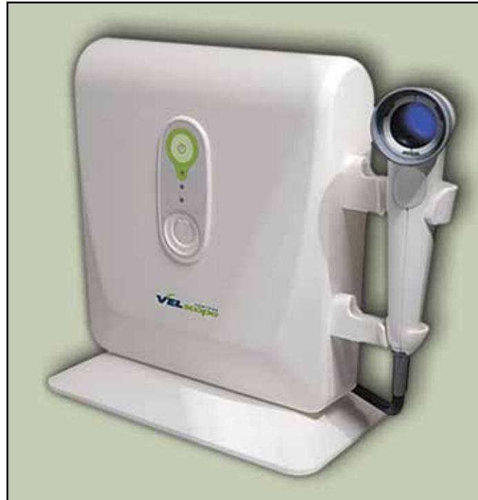
The Visually Enhanced Lesion scope (VELscope) illuminates oral mucosa with blue light but permits only green light to reach the observer’s eye. Normal mucosa appears green; lesions appear black. The current cordless VELscope Vx model is more convenient than this older bulkier version.
