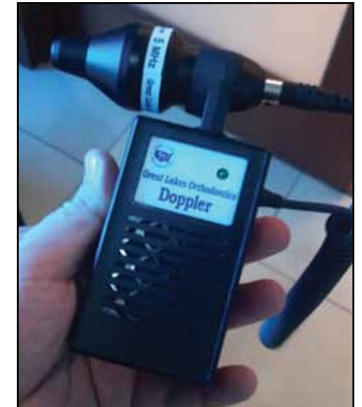
Figure 1. Portable doppler ultrasound unit which can be used to help educate patients and better document joint sounds in translation.
