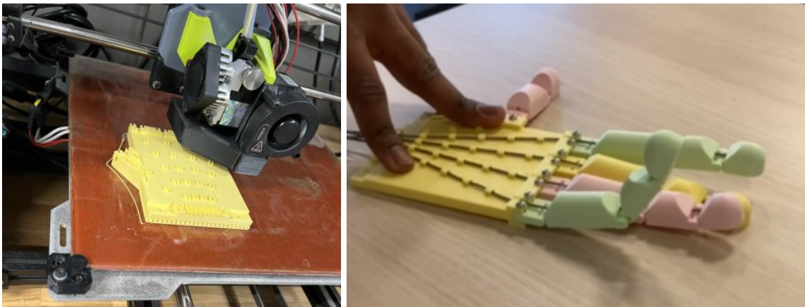
Figure 23. Early 3D printing of the hand. Images represent a prototype created during the design process.
