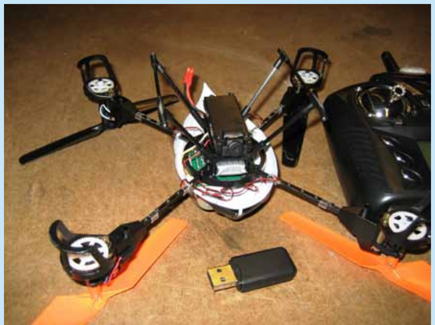
Camera of quadrotor with USB adapter for microSD card
